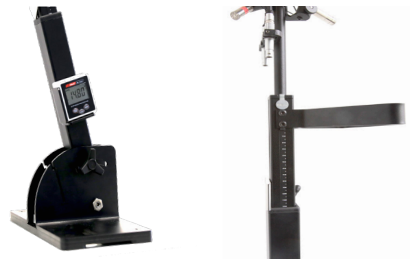
Figure 5 Angle and height indicators on the multimic microphone array.
